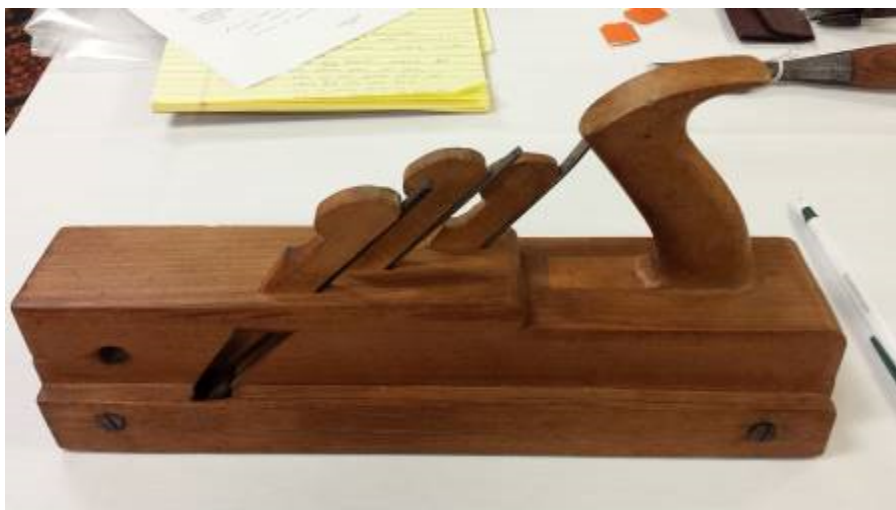
Unique 3 wedge plane by J. Coates
